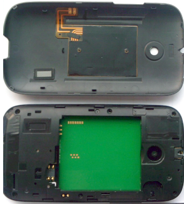
Figure 1.6 NFC antenna embedded in back cover of Huawei sonic, aka Turkcell T20.
