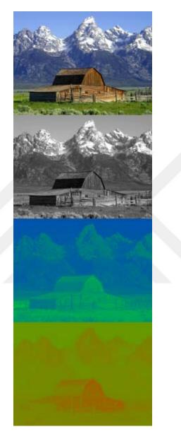
Figure 13. Image format YUV then the same image but using the Y value only then using U value only then using V value only.
