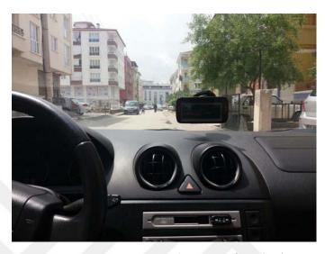
Figure 11. The M-LDWS on a Samsung Galaxy SIII functioning on a standard GPS mount.
