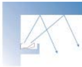
Figure 2.10: Vertical section of a cove lighting system
