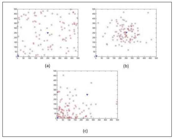
Figure 13 a. Uniform distribution of sensor nodes. b. Normal distribution of sensor nodes. c. Exponential distribution of sensor nodes. (Where o represent sensor nodes▼ represent the base station)
