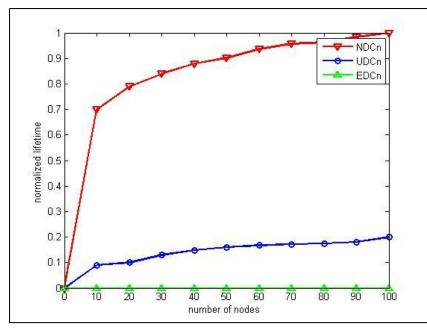
Figure 12 Network lifetime as a function of sensor node numbers (network area 500 x500 base station in the center)
