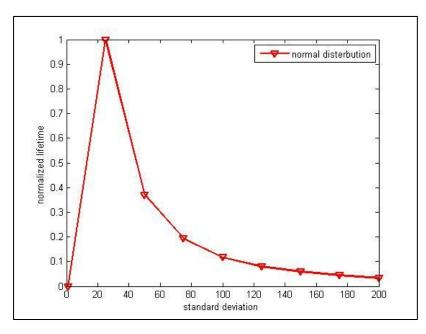
Figure 11 Normalized network lifetime as the function of standard deviation  $\sigma$
