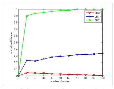
Figure 16 Network lifetime as a function of sensor node number (network area 500 x 500 base station in the corner)
