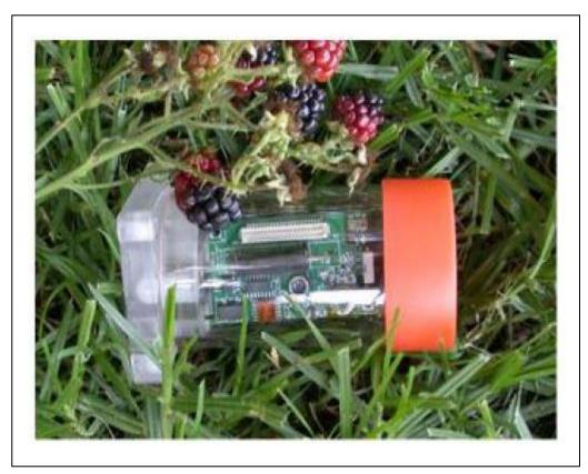
Figure 3 Deployed sensor node with acrylic fence [17]
