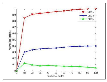
Figure 14 Network normalized lifetime as a function of number of sensor node (Network area 100 x 100 base station in the center)
