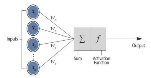
Figure 6 Typical artificial neuron node
