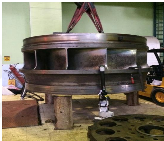
Figure 3.3 : Scanning of the turbine runner
