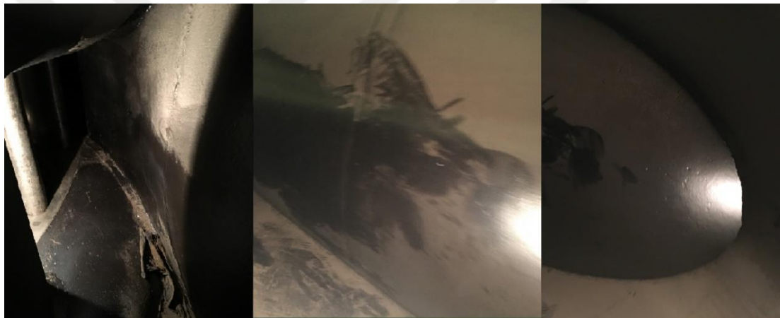
Figure 4.12: Buffer vane of the spiral Case
