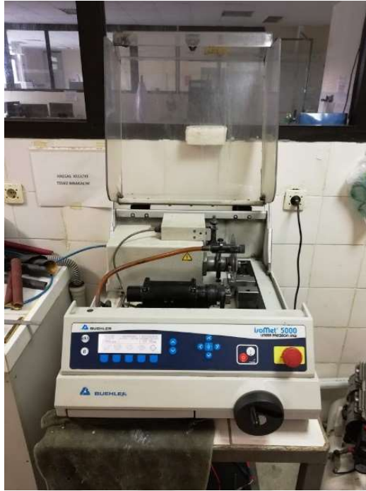
Figure 2. 7. Buehler IsoMet 5000 Linear Precision Saw device.
