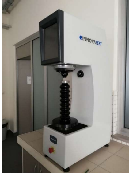
Figure 2. 6. INNOVATEST Nexus 7500TM Universal hardness tester.
