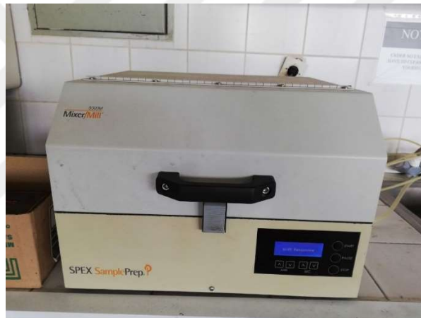
Figure 2. 4. SPEX SamplePrep 8000M Mixer/Mill ball milling device.
