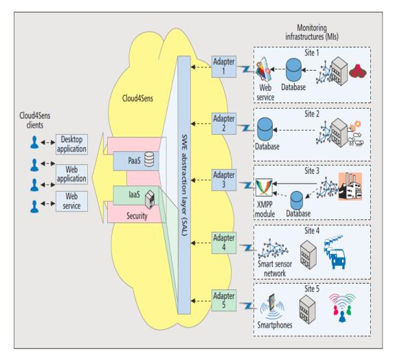
Figure (9) Cloud for Sensing Architecture [57]
