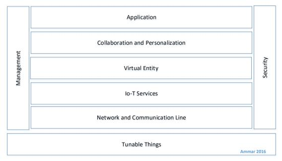
Figure (16) Web IoT Overall Workbench Structure
