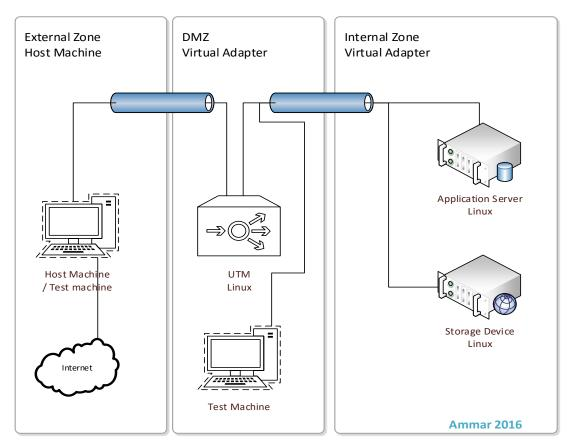
Figure (15) Test Lab Components
