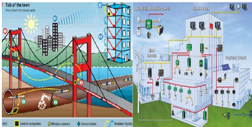
Figure 10 Applying a WSN in engineering field
