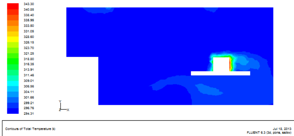
Figure 5.29 Distribution of calculation air temperature contours with k- \omega , (case 3), (a) plane at z=1.825m, (b) plane at z=0.4m
