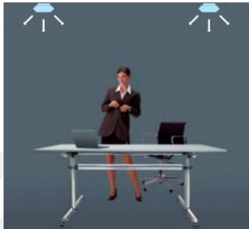
Figure 3.2a. Direct Lighting (ceiling luminaires)
