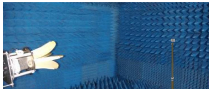
Figure 88 The fabricated of the modified antenna (a) Top view, (b) Bottom view, (c) Under VNA test (d) Measurement of radiation in the anechoic chamber
