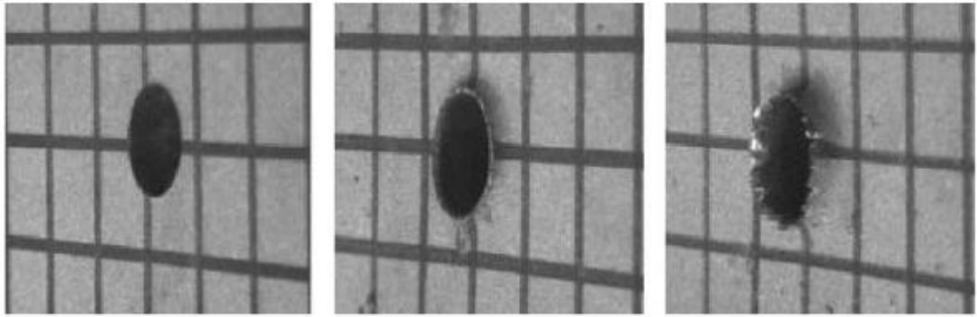
Figure 49 Real experiment's front view images are shown with blunt projectile V_0=189.4 , hemispherical V_0= 300 and conical V_0= 300.3 m/s [11]
