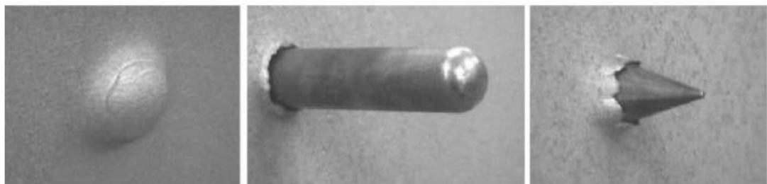
Figure 51 Real experiment's back view images are shown with hemispherical projectile V_0= 278.9 and 292.1 m/s, conical projectile V_0= 280.9 m/s [11]
