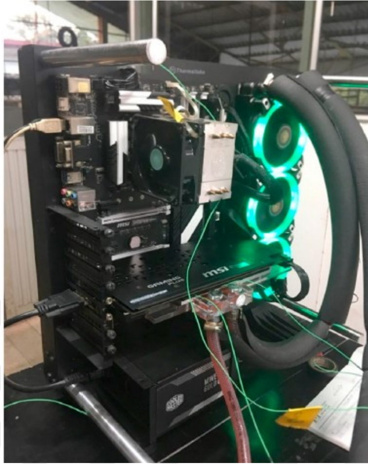
Figure 1.10 GPU attached to a heat sink with nano fluid.
