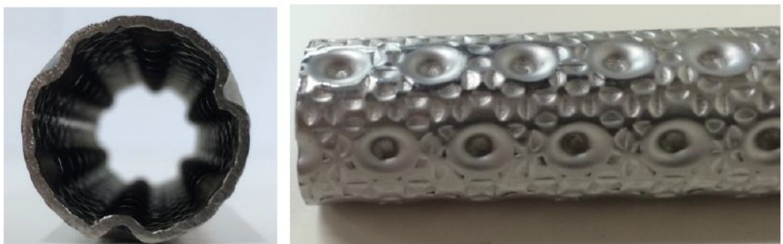
Figure 1.8 Modified tube surface using dimples.
