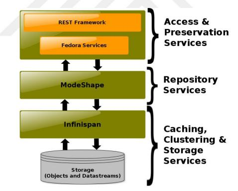
Figure 8 Fedora component stack [63]
