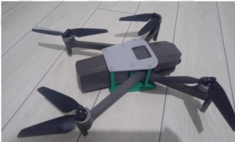
Figure 71: Designed gripper mounting assembly for quadcopter (From top)
