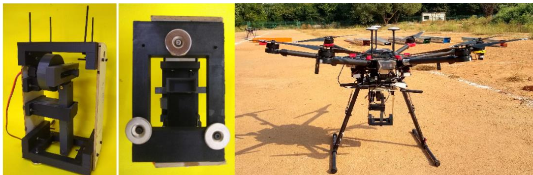
Figure 3: Drone gripper system recreated by using famous “Scotch Yoke Mechanism” [2]
