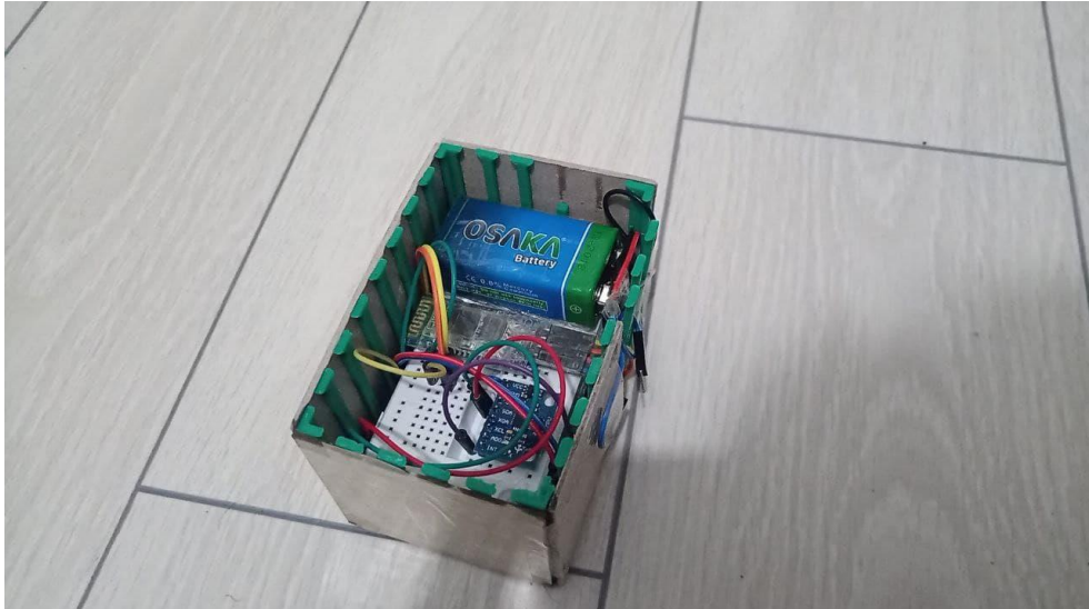
Figure 48: Cardboard box for placing Arduino circuit inside
