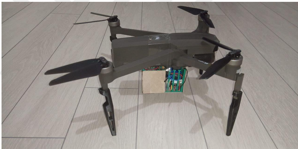
Figure 51: Prepared Arduino circuit mounted on our drone (An adhesive band has been used for mounting the circuit to bottom of drone tightly)
