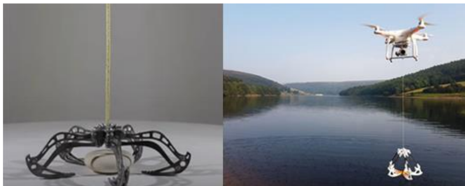
Figure 6: Self-catcher hook system mounted bottom of drone, which provide required power directly from aerial vehicle's ascending or descending motion [3][7]
