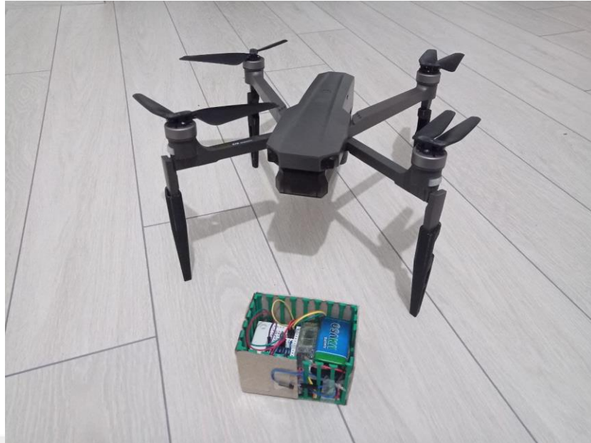
Figure 50: Prepared Arduino circuit and the quadcopter (Extra 3D printed legs made for extending drone's bottom distance from the ground.)
