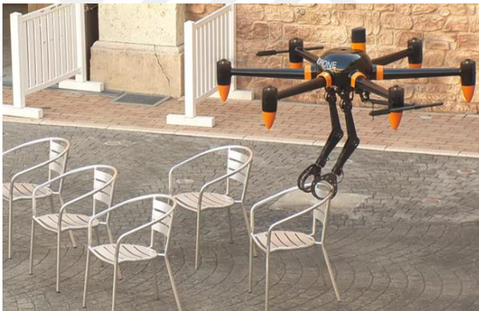
Figure 8: A motorized hybrid claw-arm system mounted bottom of drone [9]
