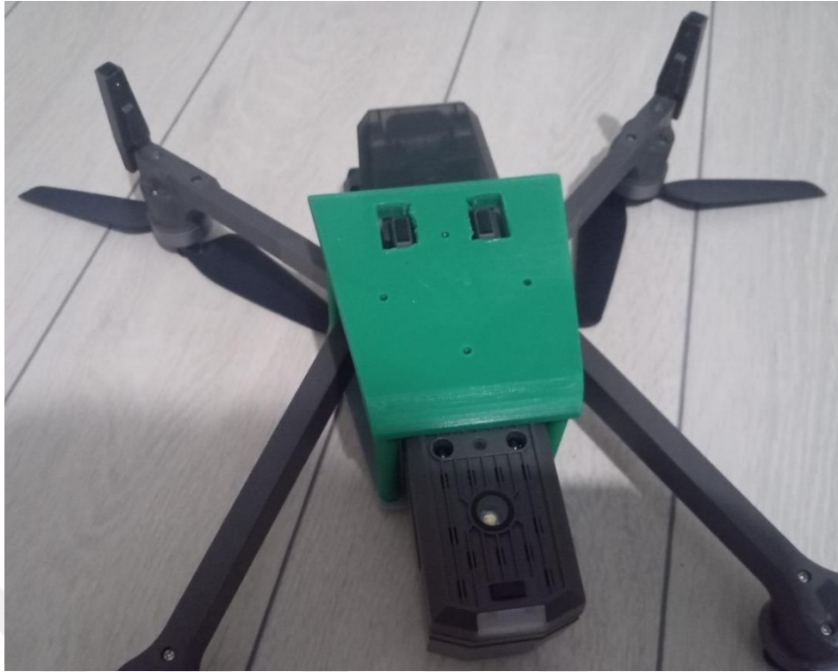
Figure 72: Designed gripper mounting assembly for quadcopter (From bottom)
