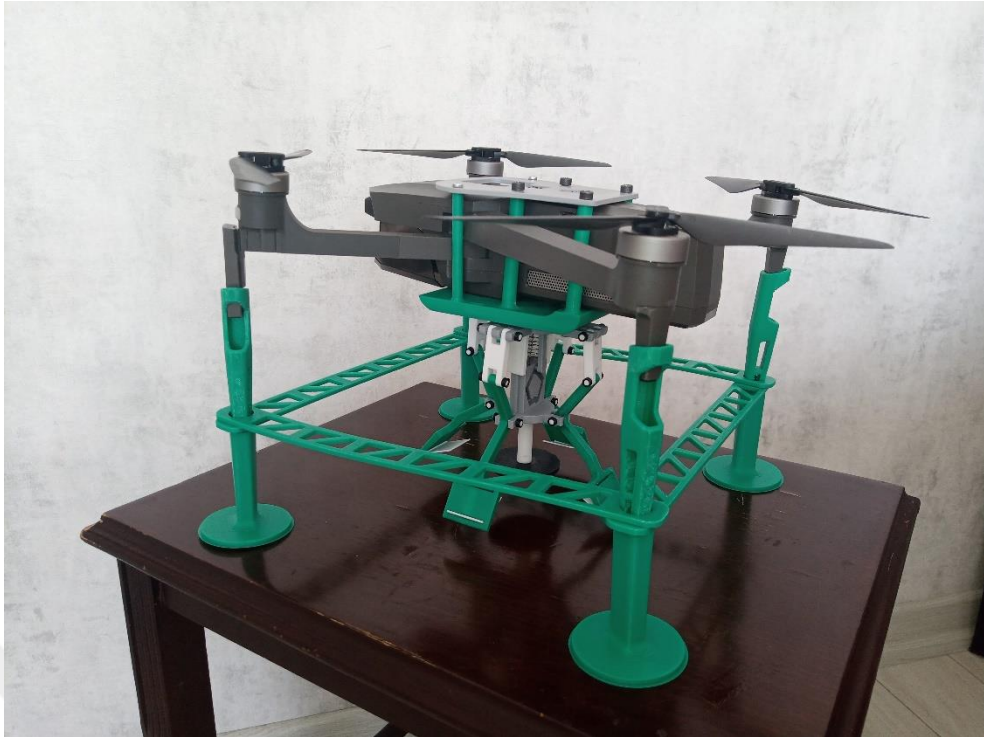
Figure 84: Created leg chassis and support beams for quadcopter and mounted gripper mechanism to middle (From front)
