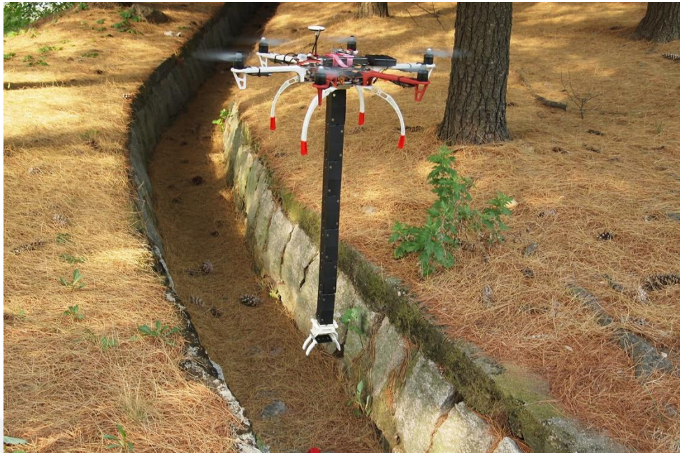
Figure 7: Origami inspired drone arm which can be collapsed or expanded in origami manner [8]
