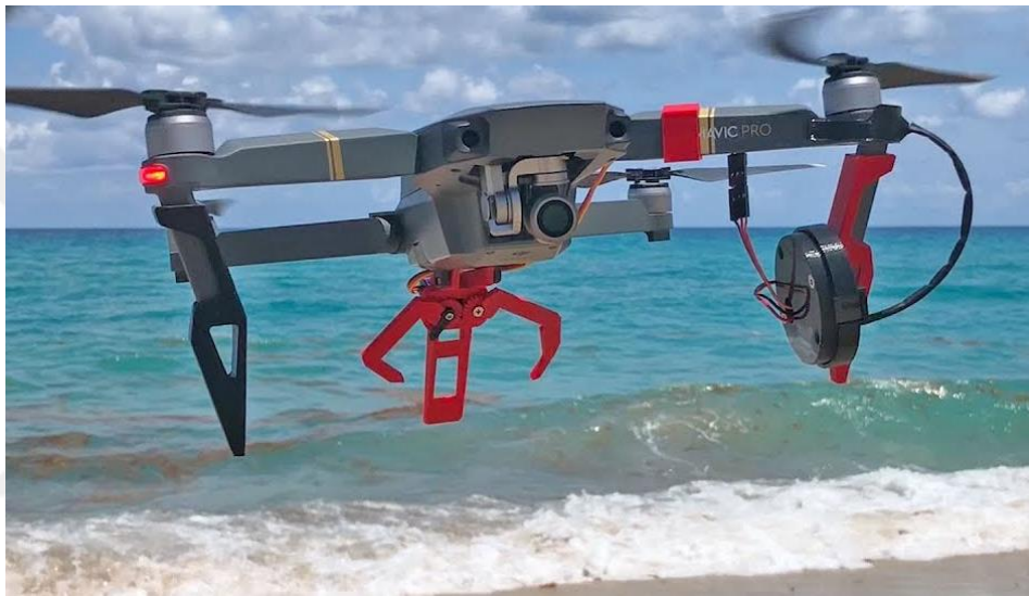
Figure 5: Motor actuated claw system mounted bottom of drone, which composed from servo motors to grasp an object [6]
