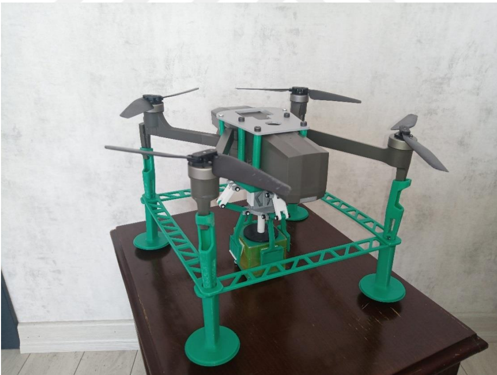
Figure 85: Created leg chassis and support beams for quadcopter and mounted gripper mechanism on middle (From back)
