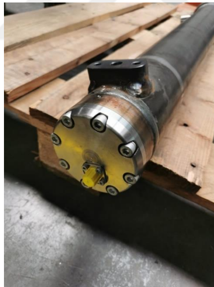
Figure 3.8: Sensor Mounted on Cylinder
