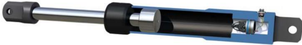
Figure 3.7: Draw-Wire Encoder Representation Mounted in Cylinder
