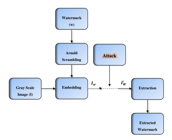
Figure 4.4: Gray Scale Image Watermarking System
