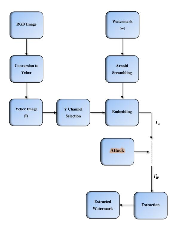
Figure 4.6: Ycbcr Watermarking System
