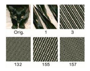
Figure 3.5: Arnold Scrambling With Different Number of Iterations
