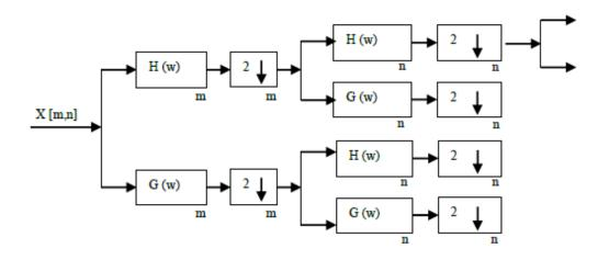
Figure 3.1: DWT for Two Dimensional Images
