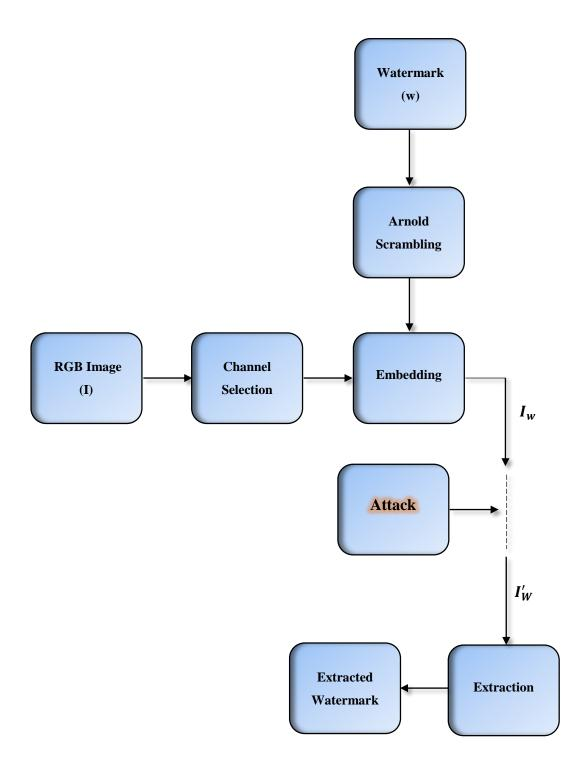
Figure 4.5: RGB Image Watermarking System
