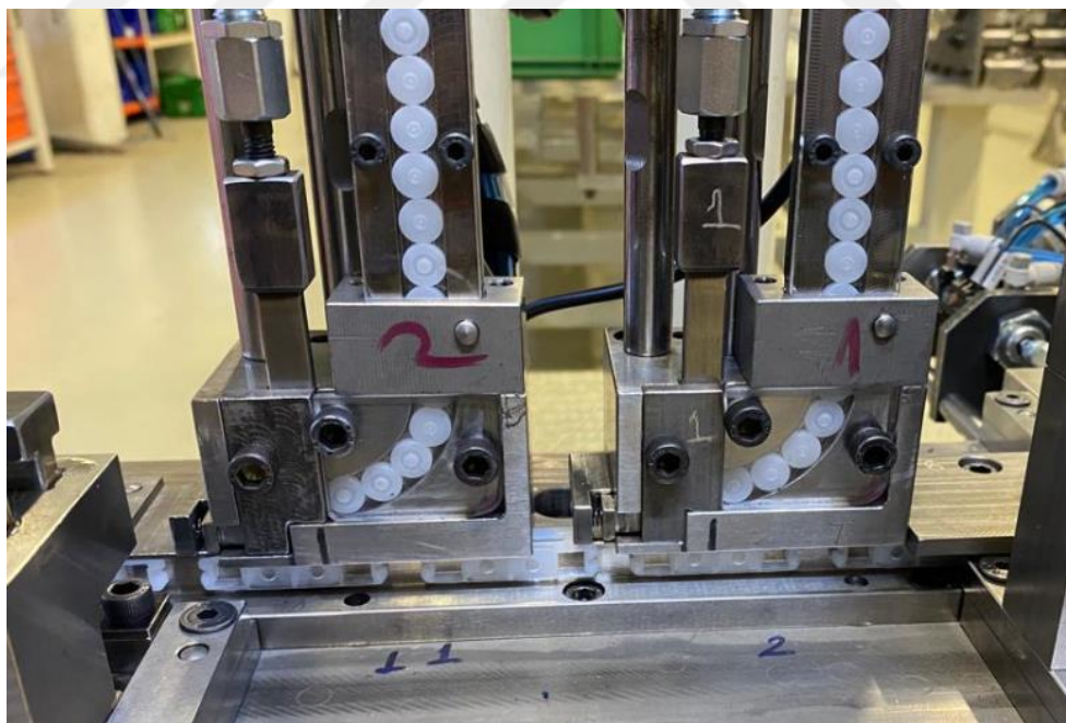
Figure 11: 1st and 2nd Ø9 mm Roller Assembly Units
