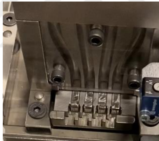
Figure 17: Design of Slide Form and Roller Guide
