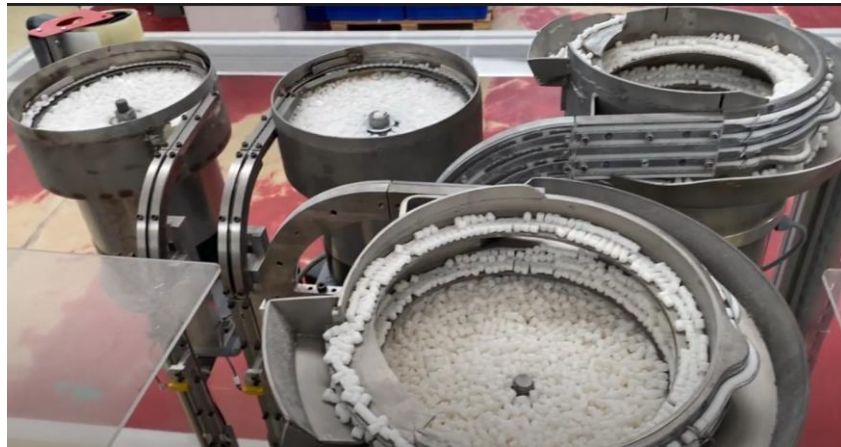
Figure 23: Vibrators of The Assembly Machine
