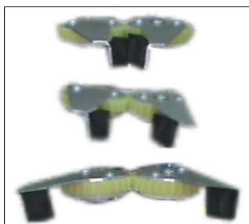
Figure 25: Arm claw from close to open state by motor “E”
