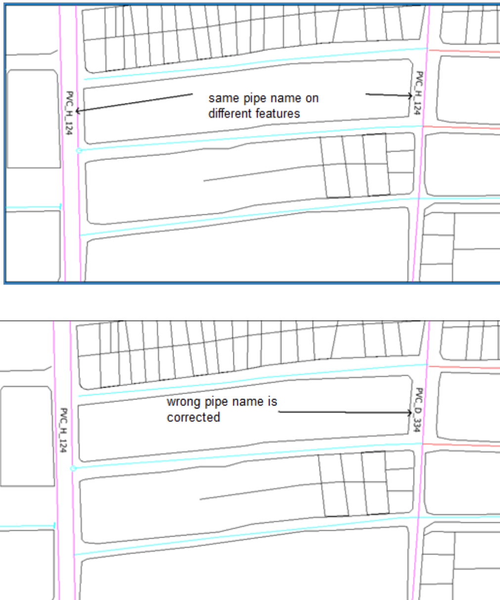
Figure 4.10 Wrong pipe names
