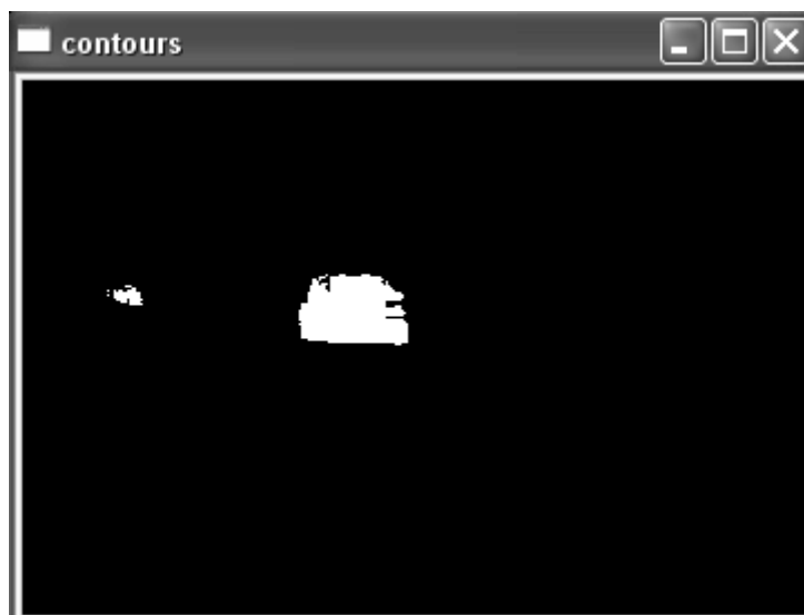
Figure 3.13: Result of the opening operation, input image is shown in figure 3.10, and 3x3 structuring element is used.
