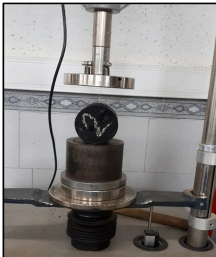
Fig. 4. Shear Resistance Using Uniaxial Compression.
