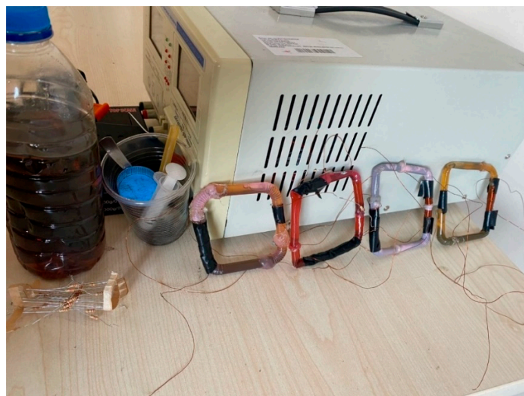
Figure 16. MFT samples with different magnetic particle mass fractions.
