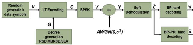
Figure 2. System model for soft-demodulation-hard-decoding approach.
