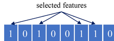
Fig. 5. The binary encoding of a solution used by wrapper-based feature selection algorithms.
