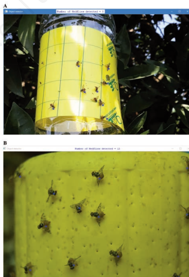
Figure 6. Trapped Medflies detected by the intelligent system, and the count is printed on the top: A) raw picture from Picbear (2020); B) number of Medflies detected.
