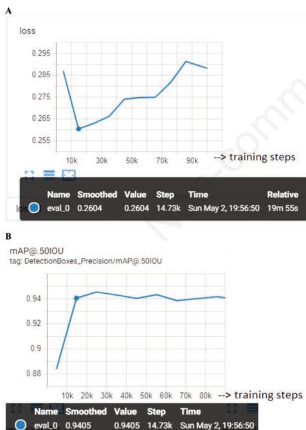
Figure 5. A) Determining the minimum loss by training the system 100K steps; B) optimising the intelligent system training process and determining the optimum mean average precision (mAP).
