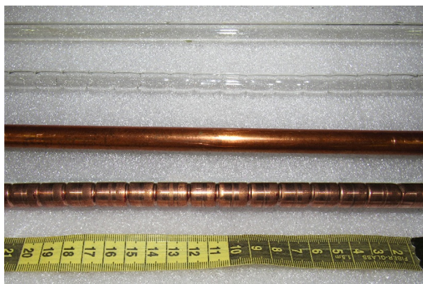
Fig. 3 Glass and copper made tubes (corrugated and smooth).
