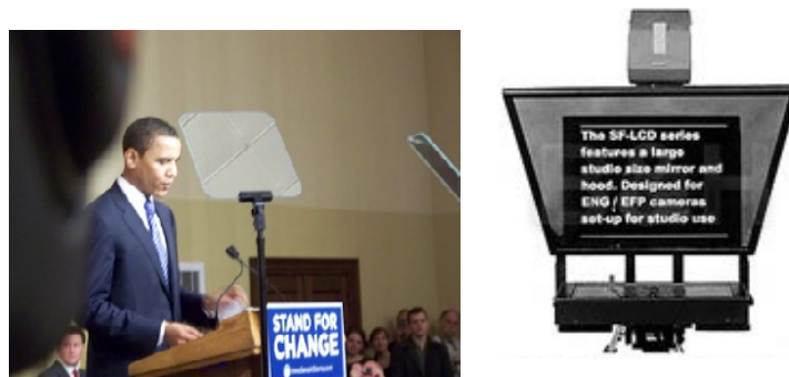
Figure 1.2: Speakers can easily read the article reflected to a transparent glass.
