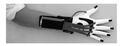
Figure 2.14: A Wearable Glove to Track the Position, Movement and Articulations of Hand [8]
