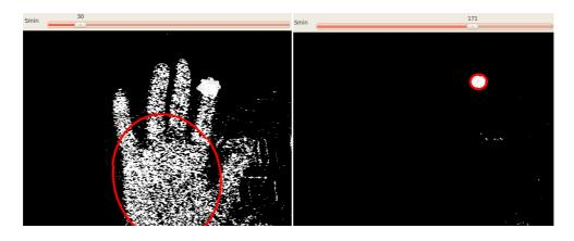
Figure 4.5: The Wrong Saturation Range and the Noise on the Left, the Correct Range with Minimum or No Noise on the Right
