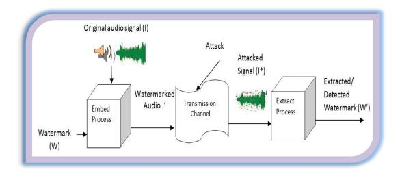
Figure 4: The watermarking system
