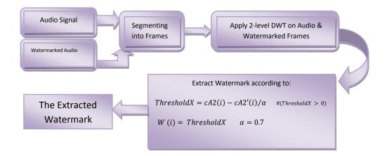
Figure 12: The proposed extraction system
