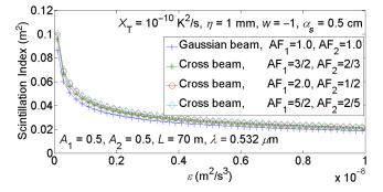
Fig. 7 Scintillation index in underwater turbulence versus  $\varepsilon$  of cross beams with individual beams having asymmetry factors, which are inverse of each other.
