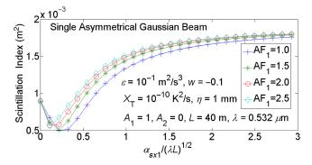
Fig. 3 Scintillation index versus the normalized source size of asymmetrical Gaussian beams in underwater turbulence.
