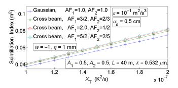
**Fig. 6** Scintillation index in underwater turbulence versus  $X_T$  of cross beams with individual beams having asymmetry factors, which are inverse of each other.
