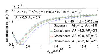
Fig. 2 Scintillation index in underwater turbulence versus the normalized source size of cross beams with individual beams having asymmetry factors, which are inverse of each other.
