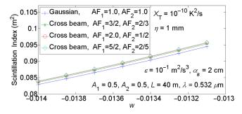
**Fig. 5** Scintillation index in underwater turbulence versus *w* of cross beams with individual beams having asymmetry factors, which are inverse of each other.
