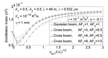
Fig. 4 Scintillation index in underwater turbulence versus the normalized source size of cross beams with individual beams having independent asymmetry factors.
