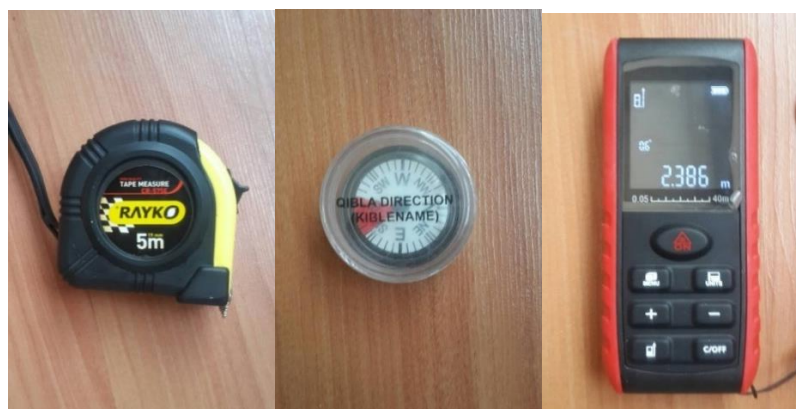
Figure 3.3: Devices used for distance, area and orientation measurements (Measuring tape, compass, laser distance measuring device)
