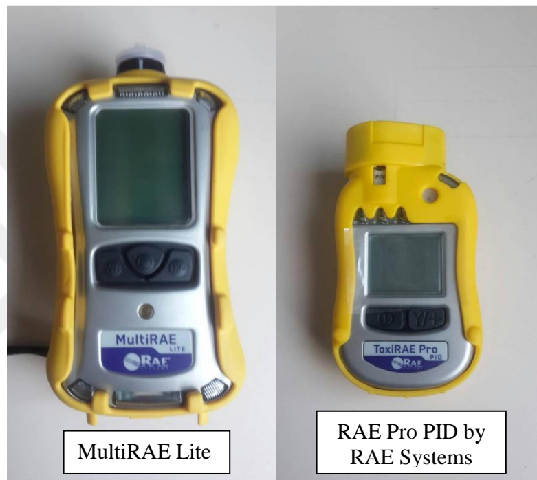
Figure 3.2: Devices used for total VOC measurement (left: RAE3775), and CO and CO 2 measurements (right: ToxiRAE Pro PGM-1800)
