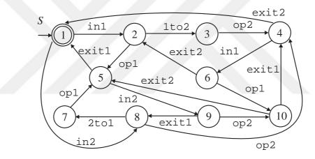
Figure 7: Maximally permissive supervisor *S* for the example system.
