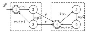
**Figure 14:** Fault-recovery supervisor *S*<sup>F</sup>.
