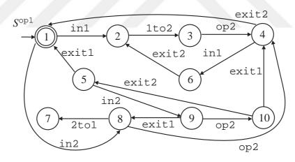
Figure 9: Closed loop with faulty event op1.
