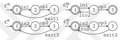
**Figure 13:** Nominal specification automaton  $C^{N}$  (alphabet  $\Sigma$ ); degraded specification automata  $C_{1}^{D}$  (alphabet  $\Sigma \setminus \{ in2, op2, exit2 \} )$ ,  $C_{2}^{D}$  (alphabet  $\Sigma \setminus \{ in1, op1 \}$ ) and faulty specification automaton  $C^{F}$  (alphabet  $\Sigma$ ).
