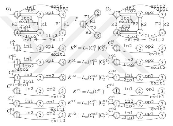
**Figure 19:** Automata models for the example system: Plant  $G = G_1 ||G_2||F$ ; nominal specification  $K^N = L_m(C_1^N ||C_2^N)$ .
