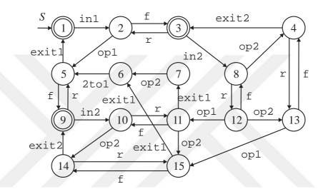
Figure 17: Supervisor *S* that solves the fault-recovery problem with system repair.
