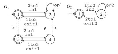
Figure 12: Plant model automata of the example system.
