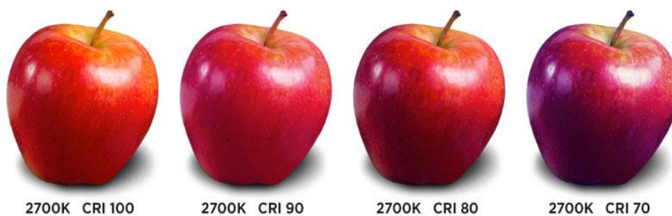
Figure 2.13: Color Rendering Index in Same Color Temperature (Westinghouse Lighting)
