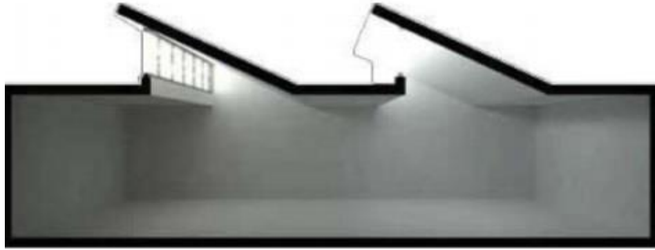
Figure 2.34: Daylight from Roof Window (Aksoylu, 2008).
