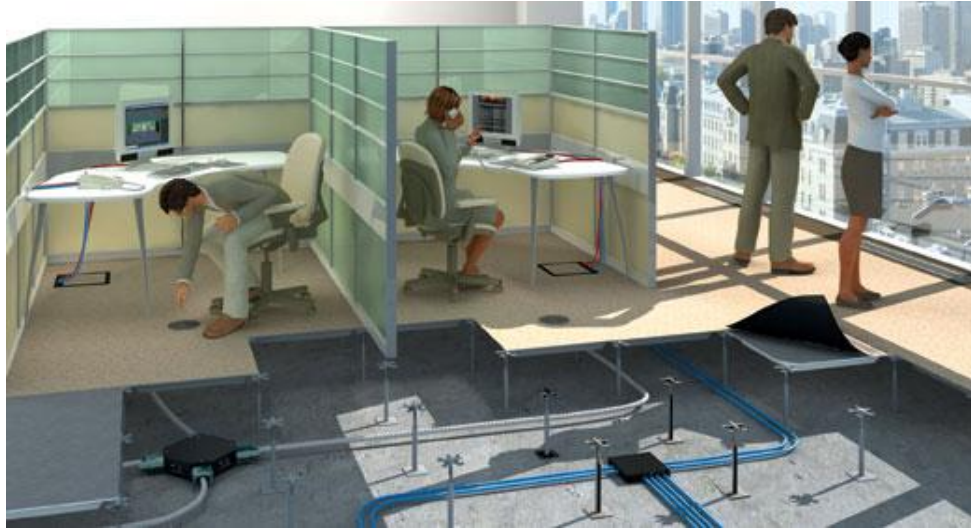
Figure 17: Raised flooring systems
