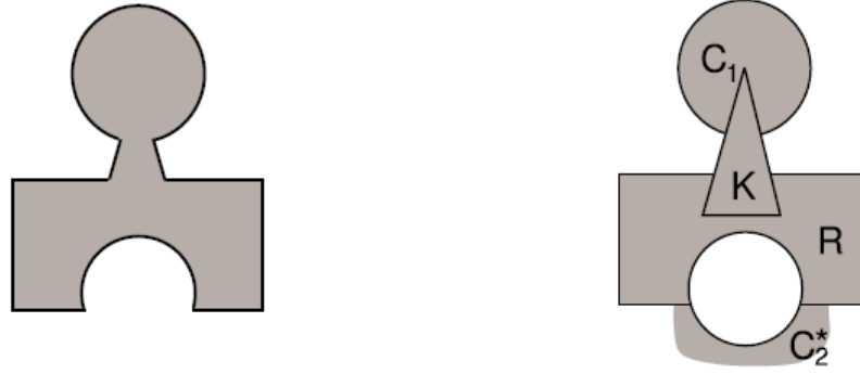
Figure 7 An example of a composed phi-object C_1 \cup K \cup (R \cap C_2^*) (Chernov et al., 2010)
