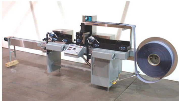
Figure 5.16 An Enveloping Machine
