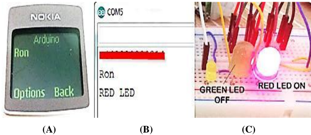
Figure 55: Manual ON/OFF LEDs testing
