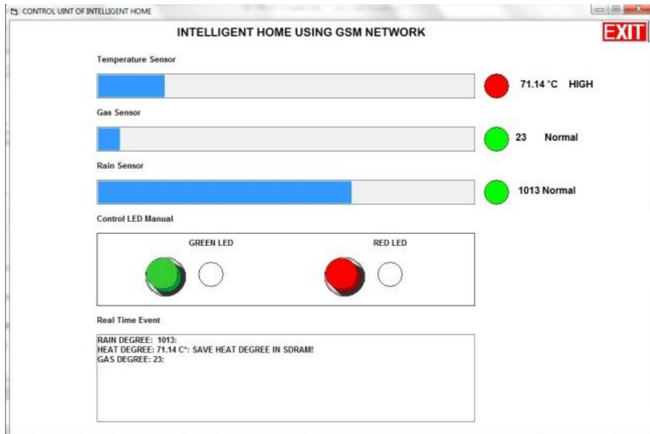
Figure 60: Software testing for increases in temperature
