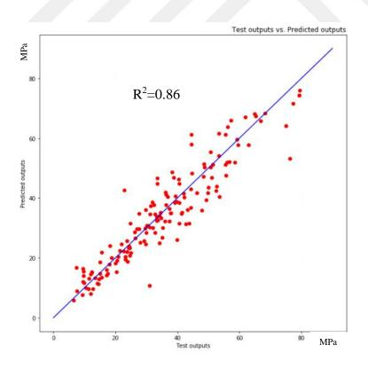
Figure 13: Test Outputs vs. Predicted Outputs for PSO-ANN Model R19
