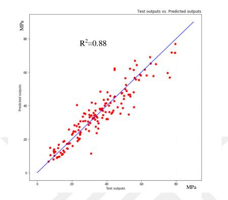
Figure 14: Test Outputs vs. Predicted Outputs for PSO-ANN Model R20
