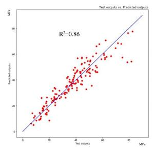
Figure 4: Test Outputs vs. Predicted Outputs for PSO-ANN Model HL7
