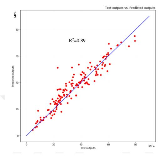
Figure 7: Test Outputs vs. Predicted Outputs for PSO-ANN Model L13
