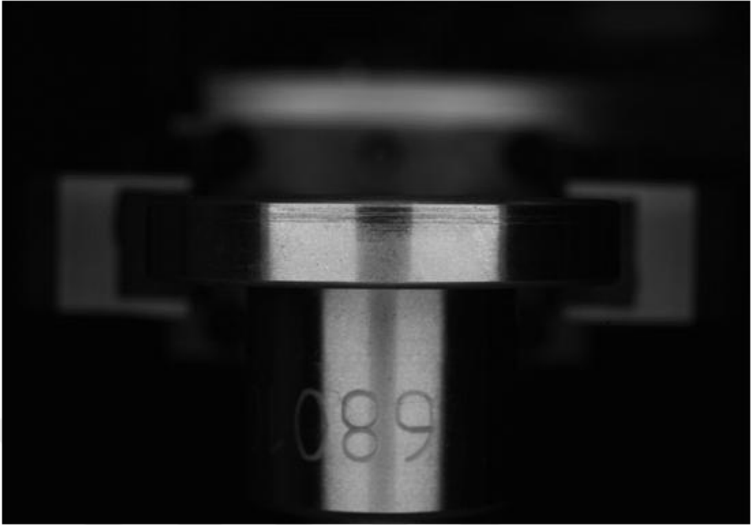
Figure 27: Example of a bearing with shoe trail defect on the outside diameter.
