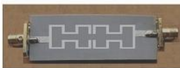
Figure 78 Graph of produced 2 nd iteration Moore fractal BPF
