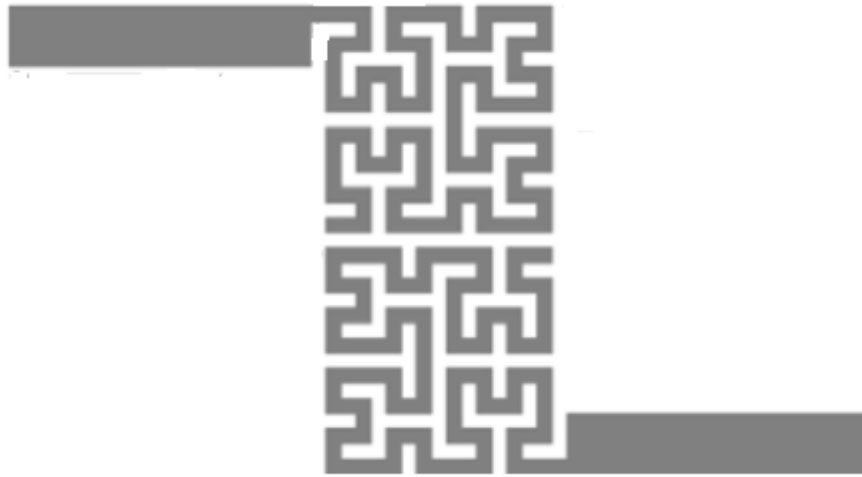
Figure 30 Typical CCSR-H based on 3 rd Hilbert fractal iteration
