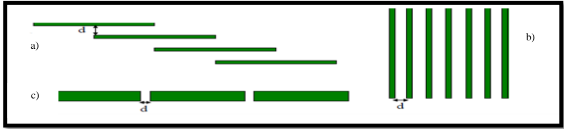
Figure 47 Basic microstrip filter layouts: a) Backward coupling, b) Forward coupling and c) Edge coupling
