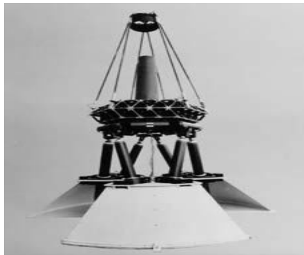
Figure 3 Vertex Antennentechnik a telescope pointing system( Hybrid manipulator)
