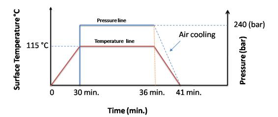
Figure 15: Optimum Parameters Plotted in Time to Explain the Operation.
