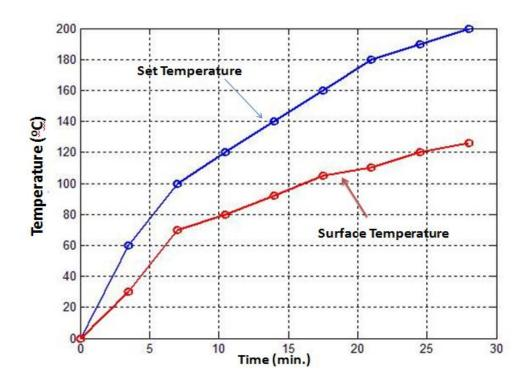
**Figure 12:** Transient Response of the Surface Temperature and the Heater Temperature. The surface temperature of the heater plate was measured with a UNI-T33C multi timer.UNI-T33C has a K type PT100 thermocouple for measuring temperature, and has a precision of 0.1°C.
