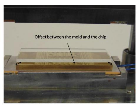
Figure 14: The Offset Between the Chip and Mold Edge
