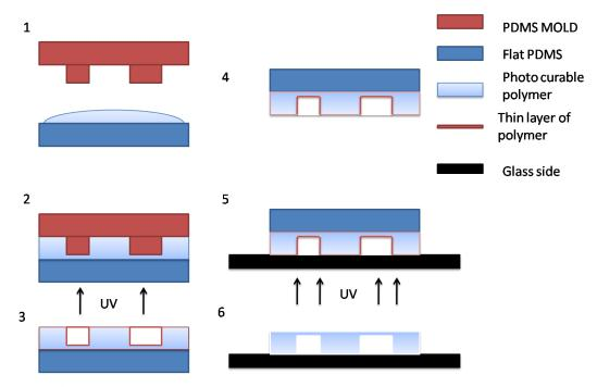
Figure 2: Illustration of Soft Lithography to Fabricate Microfluidic Chip.
