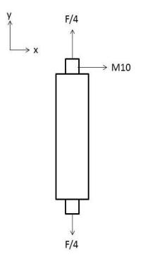
Figure: 8: Free Body Diagram of the Lower Cylinder
