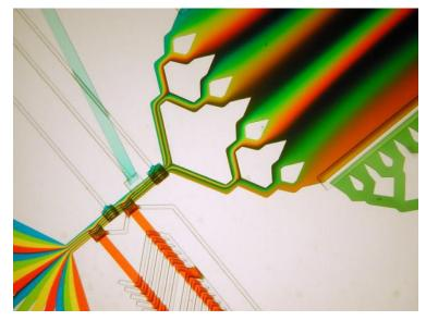
Figure 1: Part of a Microfluidic Chip Illustrating Laminar Flow and a Microfluidic Demultiplexer. Channels widths are in the order of 100 μm (Source: Folch Lab, University of Washington).
