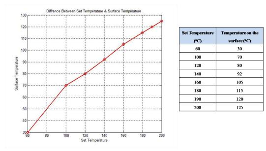
Figure 11: Surface Temperature Versus the Set Temperature
