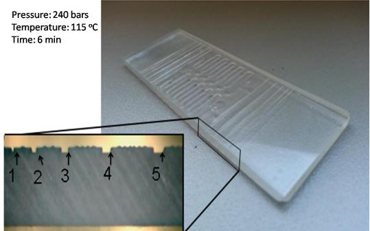
Figure 16: Patterns Obtained by Applying Optimum Process Parameters.
