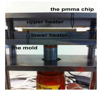
Figure 10: The way that the PMMA Chip and Brass Mold.
