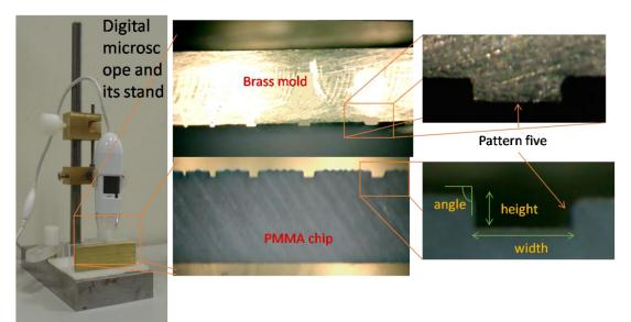
Figure 13: Use of Digital Microscope to Get the Images for the Measurements. The Measurements are Done Using ImageJ.
