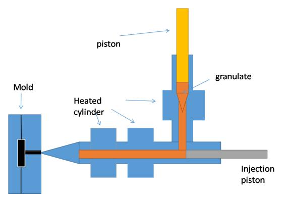
Figure 3: Illustration of Micro-Injection Molding.
