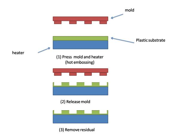
Figure 4: Illustration of Hot Embossing for Microfluidic Fabrication
