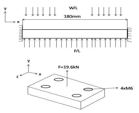
Figure 6: Loading State of the Heater Plate and Free Body Diagram of it.
