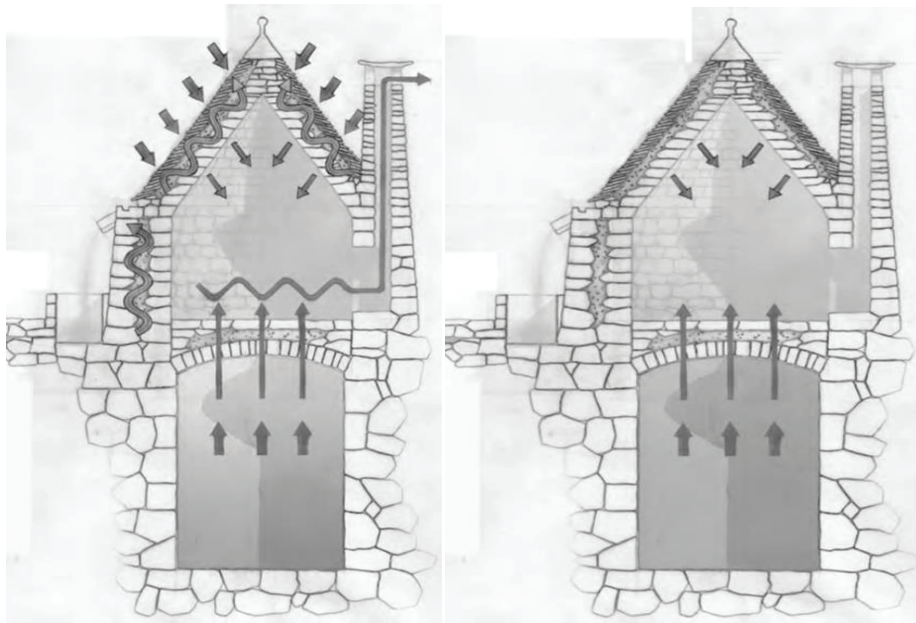
Fig. 2. The building passive behaviour. The traditional dwelling ( trullo ) thermal performance on day (left) and night (right). (Dipartimento Ingegneria Civile e dell'Architettura, 2009).
