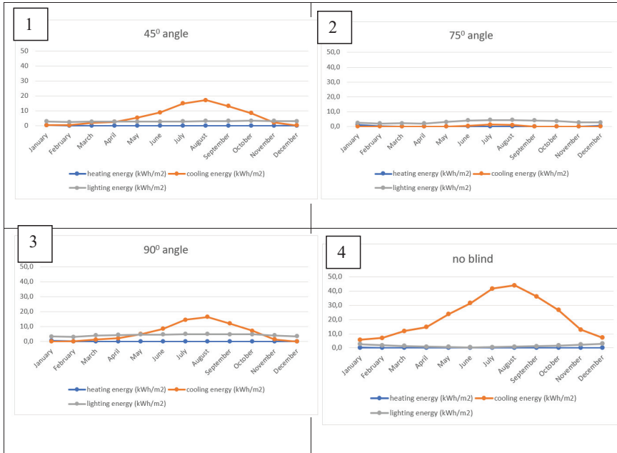
Figure 3. South facade oriented office zone models
