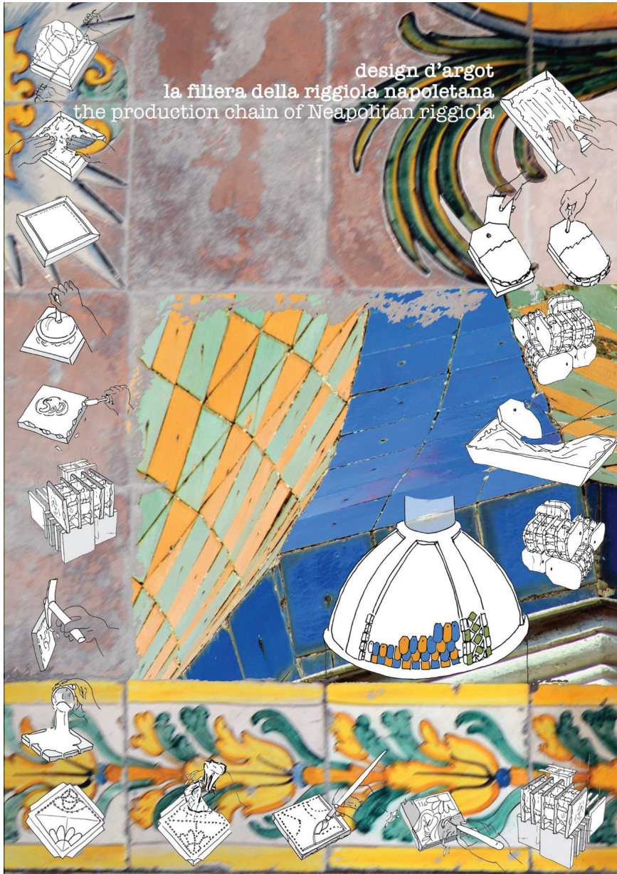
Figure 1. Argot Design : the production chain of Neapolitan ruggiola tile. From top left to bottom right, the sketches illustrate the processing sequence from raw clay to the second final firing. On the right side, there is the graphic sequence of the nailed tile for the domes.
