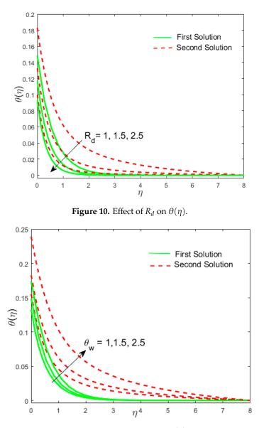
**Figure 11.** Effect of  $\theta_w$  on  $\theta(\eta)$ .
