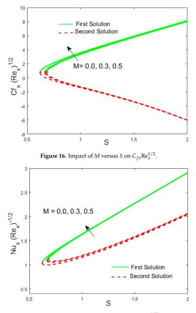
**Figure 17.** Impact of *M* versus *S* on  $Nu_x \operatorname{Re}_x^{-1/2}$ .
