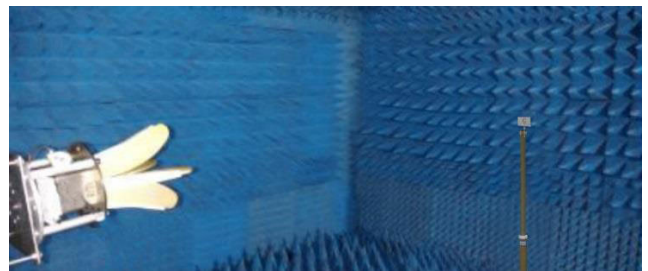
FIGURE 11. The fabricated antenna prototype in the anechoic chamber.
