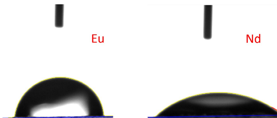
FIGURE 4 Wetting contact angle images for the Eu and Nd containing glasses
