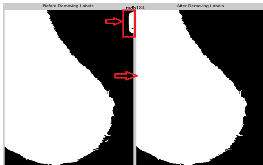
Figure 6.8 Before and After Removing Labels
