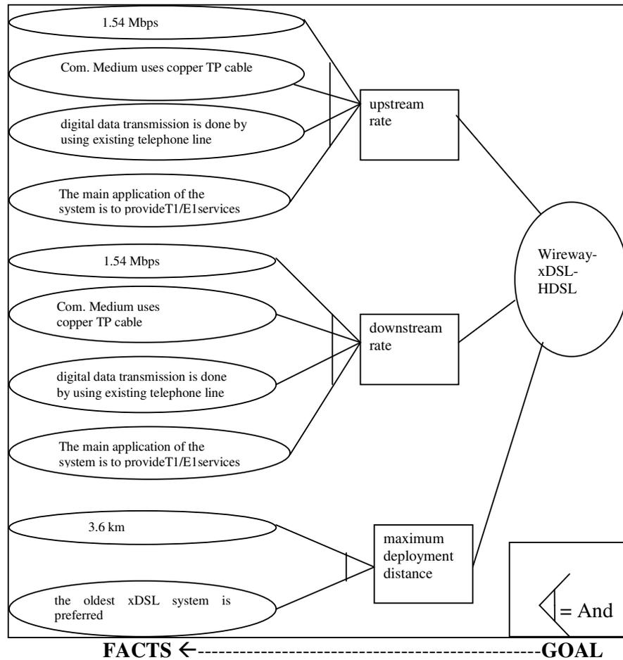
**Figure 2 :** Example AND --- OR Logical Representation Of Rule 8, Rule 44, Rule 96 For The Optimum Access Telecommunication Network System Decision With Backward Chaining Inferencing
